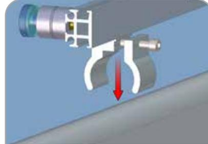
Once graphic is attached to stand-offs and extrusion, position tube clamps (TC-30) onto backwall.
