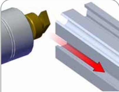
Before attaching to graphic, slide end of stand off (CKSO) into extrusion. Repeat for other stand-off(s).
