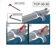
Using provided 5mm hex key, rotate bolt clockwise to secure accent to top of fabric backwall.
