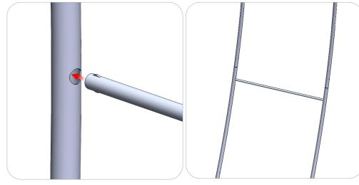
Locate the spreader with rounded clips on each end. Simply push each end of the spreader in any orientation into the holes of the center tubes in your bungee assembly. There is no need to supress the clips by hand.
