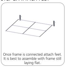
Use provided allen key, secure feet to bottom of frame by screwing bolt.
