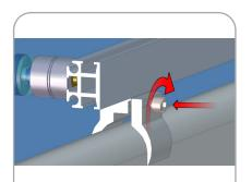
Using hex key turn bolt clockwise to tighten tube clamps, securing graphic header to backwall.
